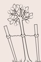
Problems with staking Stakes bent, wires loose, tree not secured
