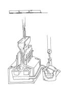
**6.** The lids are fed through a high precision process where rivet making, scoring, and tabbing occur in consecutive operations.
